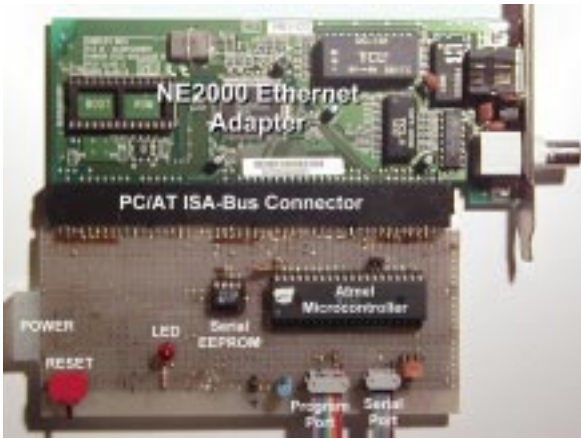
Photo 1 —Here's the PicoWeb server breadboard with a $9 ISA-bus network card and an Atmel AT90S8515 8-bit microcontroller. Connectors at the bottom provide a serial port and an in-circuit programming port using a PC parallel port cable. Power (150 mW typical) is supplied by a +5-VDC wall wart.
