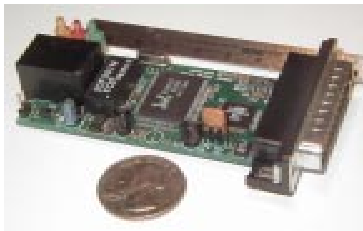
Photo 3 —Here's the fully integrated PicoWeb server.
